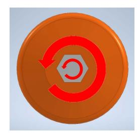
Here, the wheel and the shaft are connected in the same way, but with a hex shaft.
