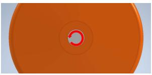
However, the wheel does not rotate because the cylindrical shaft is loose in the cylindrical bore of the wheel.
