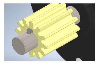
Figure 5: A pinion connected to a motor by a key, the small darker-colored part between the gear and the shaft
