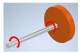
A wheel is connected to the shaft. As it rotates at one end, the other end of the shaft rotates, too.
