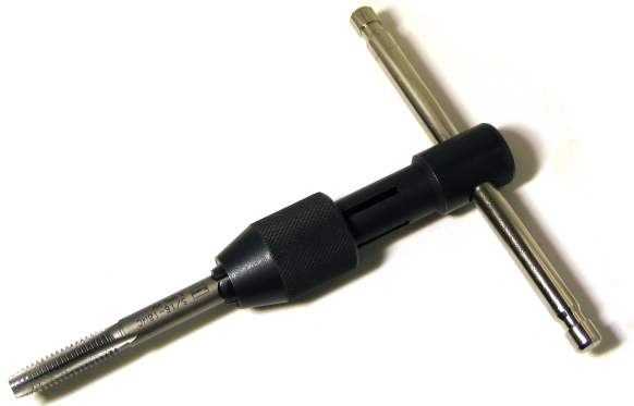
Figure 1: Tap and handle. The handle is turned to cut threads into the hole, much like driving a bolt into hole. (image from Wikipedia.org )
