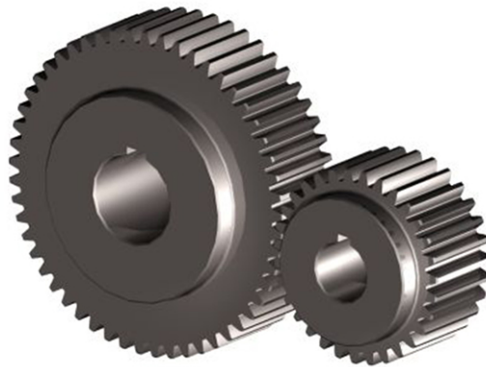
Figure 1: Two interlocking spur gears. Note how the teeth lock together (Image from MotionControlTips.com )
