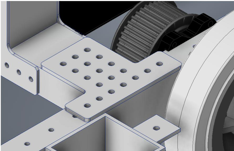
Figure 7: A gusset on the 2019 robot which uses a rivet pattern. Each rivet is 0.5" from the next one in all directions. Note that the rivets are not modelled in CAD.
