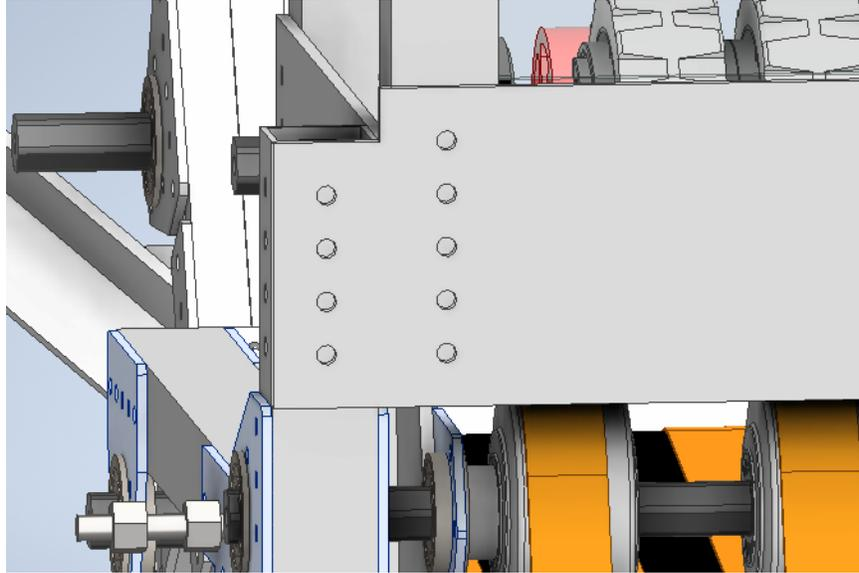
Figure 9: Match drilled holes on the 2017 robot. The holes are only modelled in the flat piece in front, not in the tubes.
