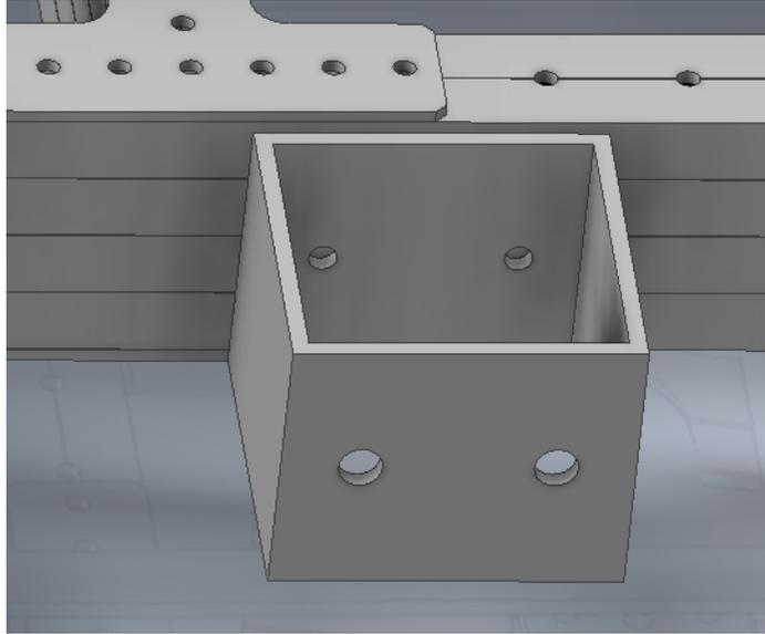
Figure 8: A bumper mount on the 2017 robot, with only two bolts used in the joint. Note that, again, the fasteners are not modelled
