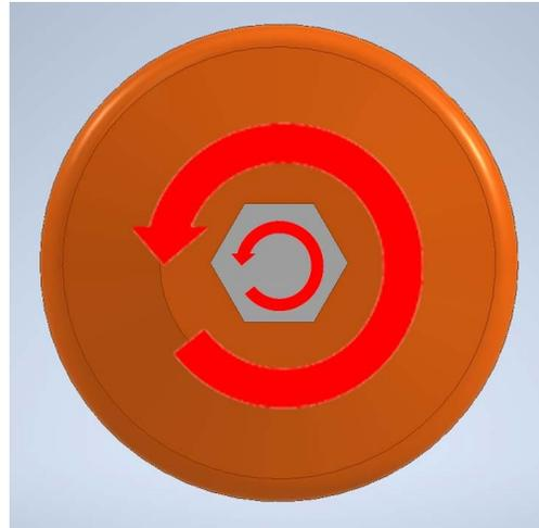
As the hex shaft rotates, the wheel rotates with it.
