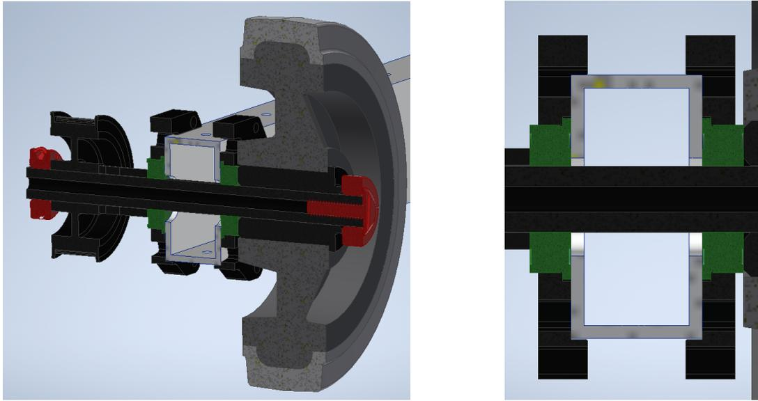
Figure 5: Section view of a drivetrain shaft assembly from the 2018 robot. In this case, the flanges of the bearings are constrained in both directions, held between the frame and the bearing blocks, the large black pieces on either side of the frame.
