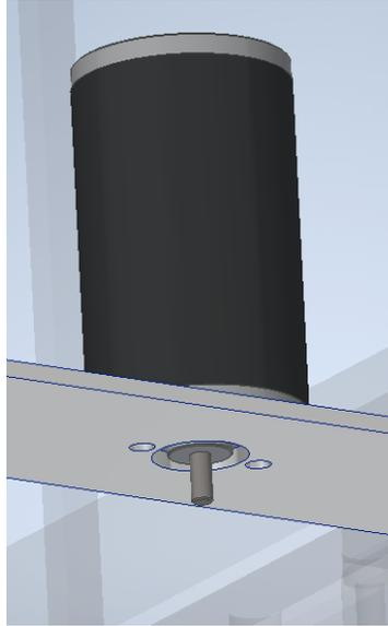
Figure 1: A BAG motor mounted to a flat bar on the 2019 robot. The holes are for bolts which are not modelled, and a pulley on the output shaft is hidden.
